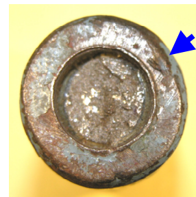
Fig. 1b Magnified view of the broken tie rod showing dent mark and bright fracture surface
