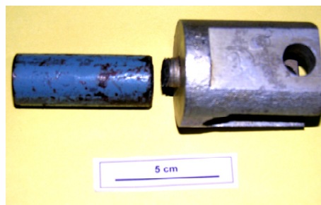
Fig. 1a Photograph showing as received condition of broken fork end and tie rod of frame.
